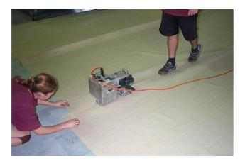
Welding of materials is also carried out by thermal welding using hot wedge welders. Thermal welding can be carried out on a large range of materials including shadecloth. Hot wedge welding can also provide watertight seams along with added strength compared to sewing. The traditional method of sewing of materials is of course still used and with developments in thread technology over the years, products have been able to achieve better life expectancy without the need for restitching.
